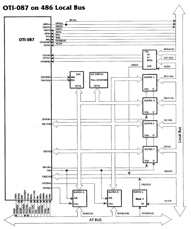
Note 1: Buffer G is needed only if the system chipset does not route back these address signals during DMA/Master cycles.
